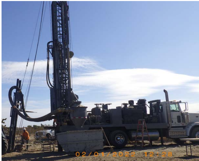
Speedstar 50K rotary drill rig configured for ARCH
